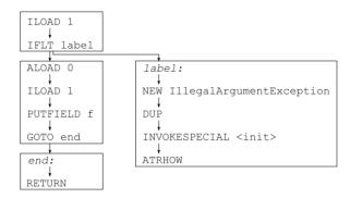
This graph can be decomposed in four *basic blocks* (shown above with rectangles), a basic block being a sequence of instructions such that each instruction except the last one has exactly one successor, and such that no instruction except the first one can be the target of a jump.
