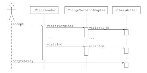
Figure 2.7.: Sequence diagram for the ChangeVersionAdapter
