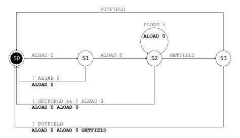
Figure 3.6.: State machine for ALOAD O ALOAD O GETFIELD f PUTFIELD f
