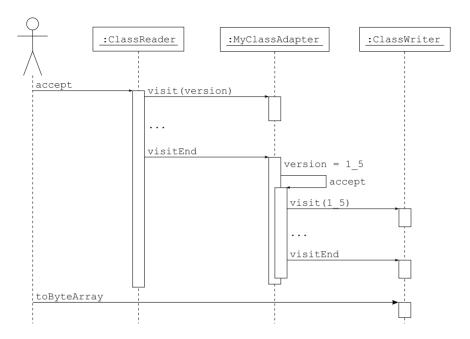
Figure 6.2.: Sequence diagram for MyClassAdapter
